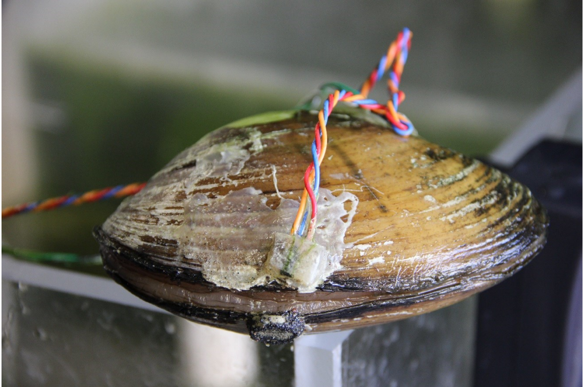
Figure 3.8 Experimental placement of hall sensor and rare earth magnet on freshwater mussel.
